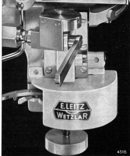
The illustration shows the freezing stage with CO 2 connection.
